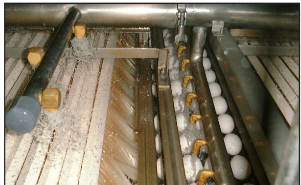
Egg washing machine in operation in the USA
